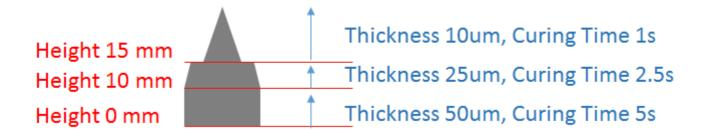
Set different Thickness and Curing Time parameters in three interval. Variable Slicing will be executed when you choose this mps file.
